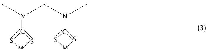
Therefore these new flocculants could remove not only turbidity but also various species of heavy metals in water. Here these
