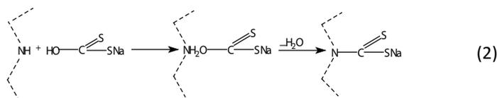
The new kinds of flocculants synthesized in such principle have the function of trapping heavy metals through chelation reaction as shown in follows.
